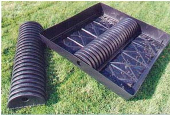
The EPIC irrigation system is a product of Rehbein Environmental Solutions. The irrigation system is based on the surprisingly simple concept of collecting all water and storing it safely below the ground. A blanket of 4x4 foot plastic cells, connected by piping, is installed across the length of the field. This is covered by 10-12 inches of sand with turf laid on top. Pipes supply the plastic cells with a constant reservoir of water. Any runoff water from rain gutters and
